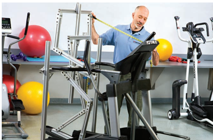
NO SWEAT Project leader Peter Anzalone designed this device to test the ergonomics of elliptical machines. It represents the range of statures of adults in the U.S.
